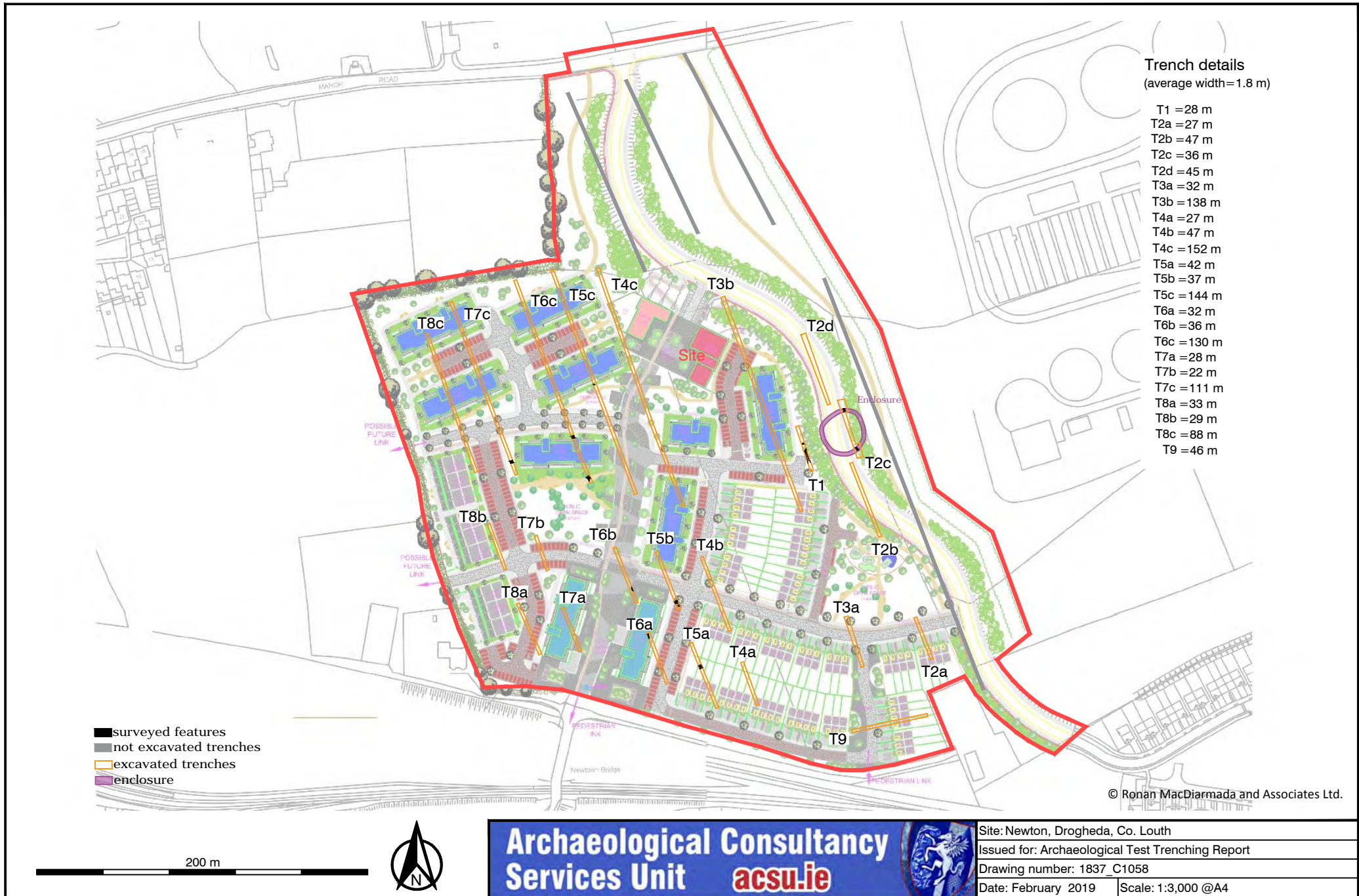
Figure 8: Plan of excavated test trenches overlaid on proposed development
